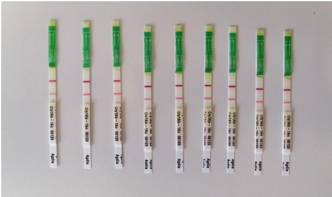
Figure A4. The ImmunoStrip test used to check whether the Bt plants used contain Bt . This test, produced by Agdia Inc., is intended for qualitative determination of Bt-Cry1Ab/Cry1Ac proteins in corn and cotton seed and leaf tissue. Here each plant tested is containing Bt .
