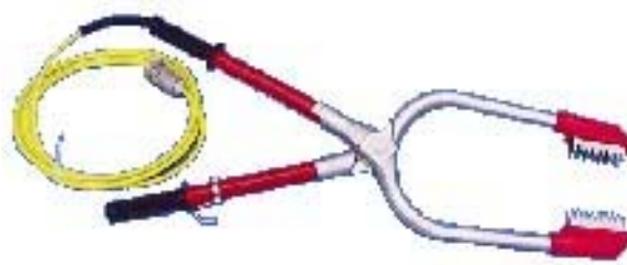
Figure 5. Scissor-type stunning tongs.
