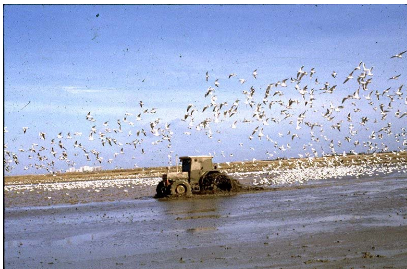
Figure 2.6.4. One of the more important works in the Flooded Paddy rice fields is done with special rotovator machines.
