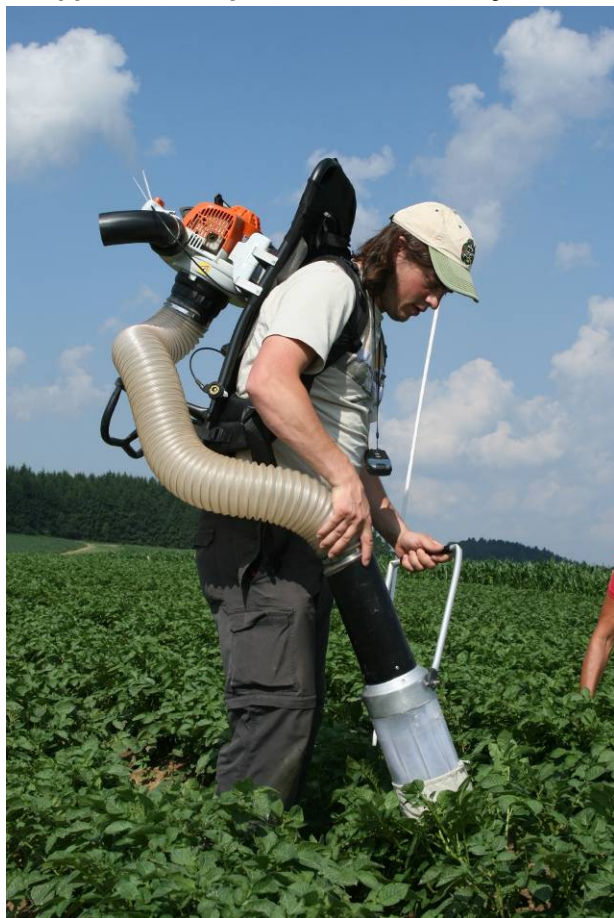
Appendix 7: Suction sampling of phytophagous arthropods with a D-Vac suction sampler
