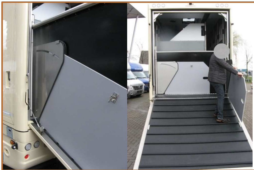
Figure 3.1 Side protections on a horse truck
