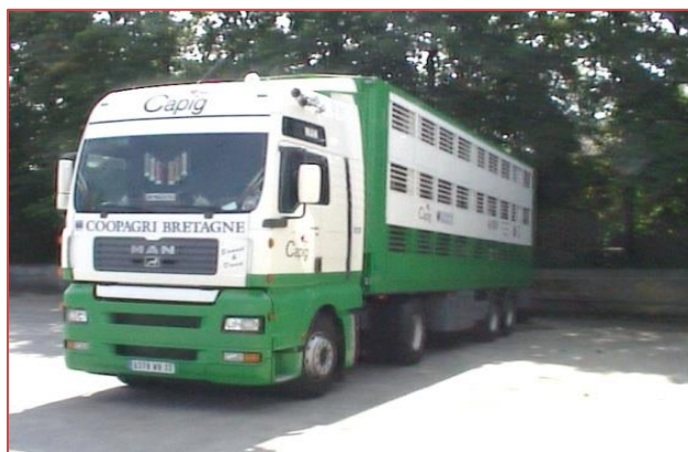
Figure 4.1 In hot weather, trucks should be parked in the shade, with lateral flaps or shutters fully open to allow free circulation of air inside the pig compartment. The ventilation system, which must be available on trucks for long-distance transports, should always be activated during stops.
