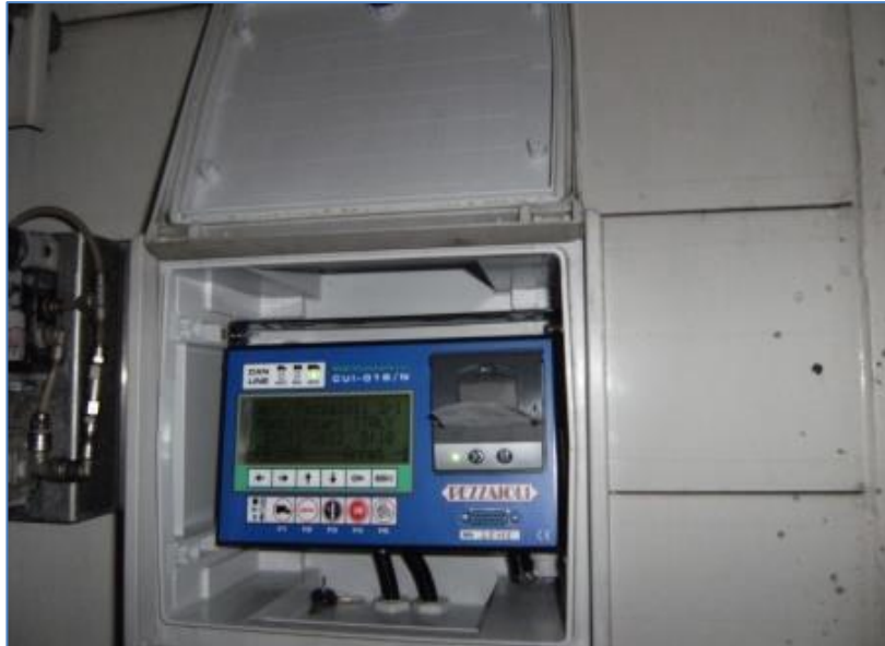
Figure 4.3 Climate controlled vehicles with automatic monitoring allow for easier and more precise adjustment of temperature and ventilation parameters inside the livestock compartment.
