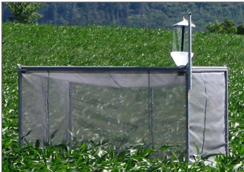
Figure 2: Light-trap cage (A). The trap is joined to the cage with a funnel. Large number of ECB will be attracted, fall down and lay eggs on the maize plants within the cage.
