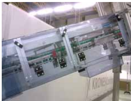
Preform conveyor covered to protect from contamination
