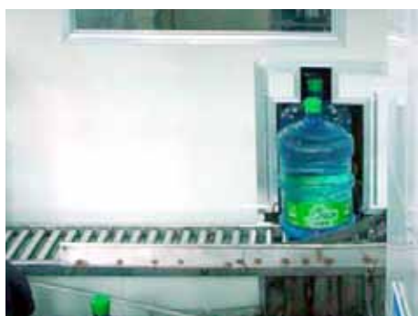
Conveyor opening adapted to the size of the container
