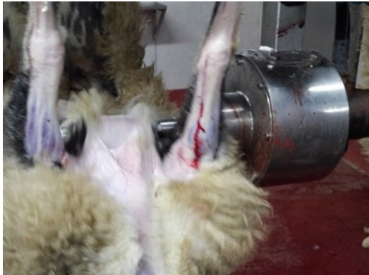
Photo : Mechanical rollers can roll the breast pack hygienically
