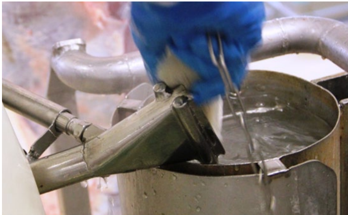
Photo : brushing the cleaning head with hot water
