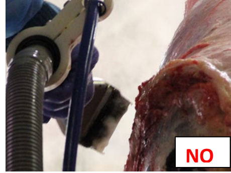
Photo: Proper positioning of the cleaning head, properly adhering to the surface of the carcass
