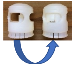
Photo: the weasand was sucked and blocked into the windows of the plug
