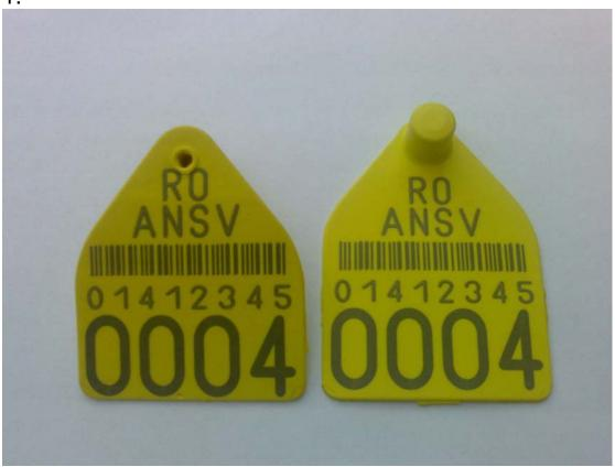
For the printing of the barcode on this model, system "interleaved 2/5" is used. The reading of the code with the barcode reader is only numbers (the 12 numbers from the identification code of the animal and printed below the barcode, without ISO code of the country) and the check digit is read last, but on the printed numbers the check digit is the  $3_{\rm rd}$ .
