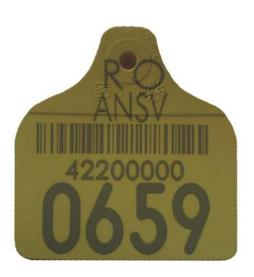
For the printing of the barcode for this model, systems "128" is used. The code read with the barcode reader is exactly the identification code of the animal (RO+12 numbers) where the check digit is the  $3_{rd}$  number. For this model the check digit is calculated with algorithm Modulo 7.
